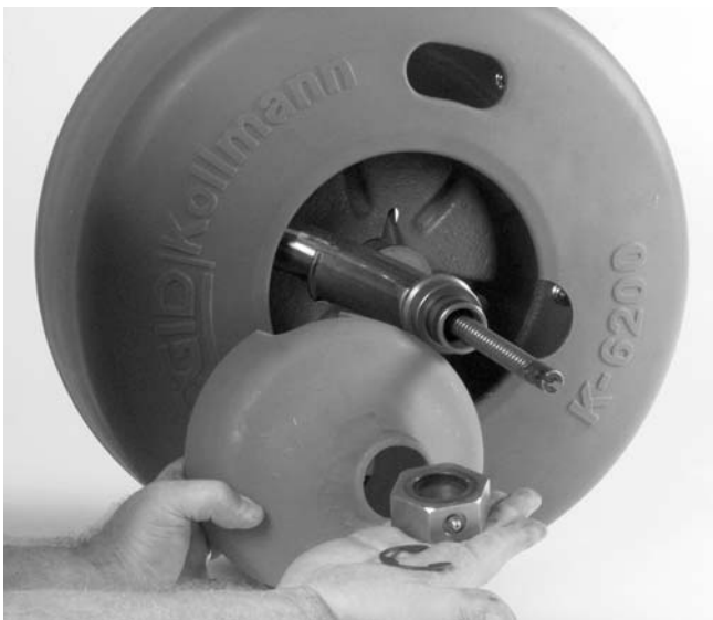
Figure 13 – Remove Retaining Ring and Inner Drum
