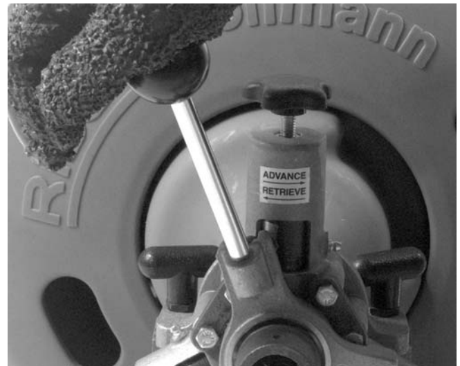
Figure 9 – Feed Lever Operation
