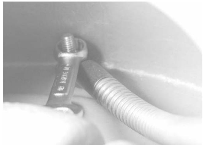
Figure 14 – Removing Pigtail Anchoring Bolt
