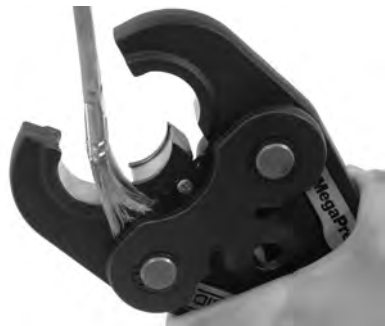
Figure 13 – Cleaning Segment Area of MegaPress Jaw
