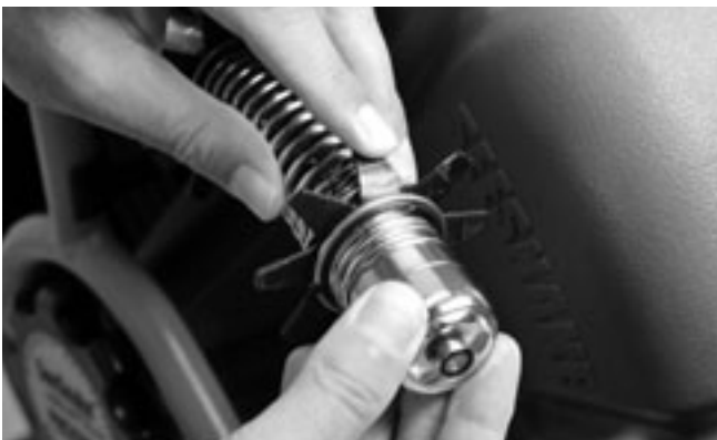
Figure 14 – Pre-stressing The Flanges
