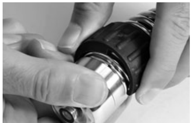
Figure 34 – Turning Camera Head Off The Spring With Spring Wrench
