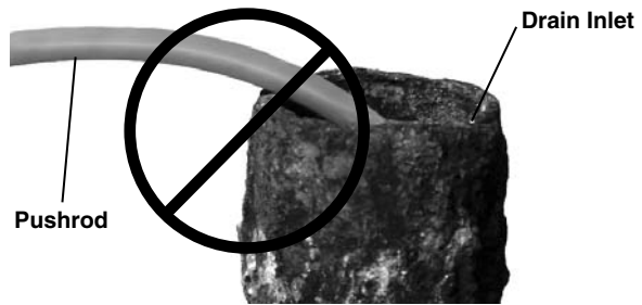
Figure 23 – Avoid Pulling At Sharp Angles
