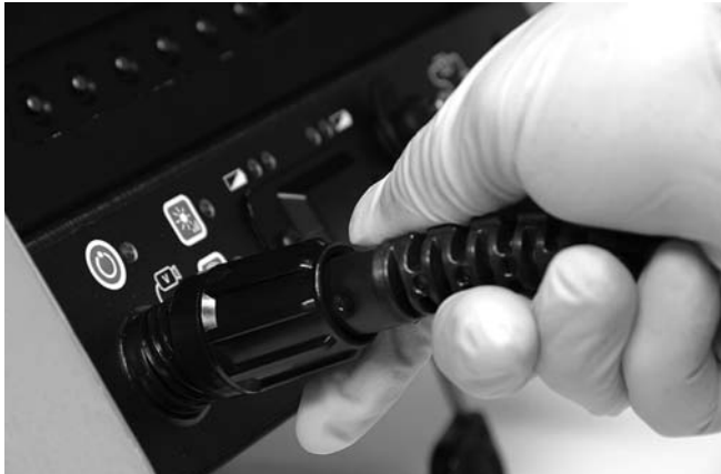
Figure 17 – Connecting To A SeeSnake CCU
