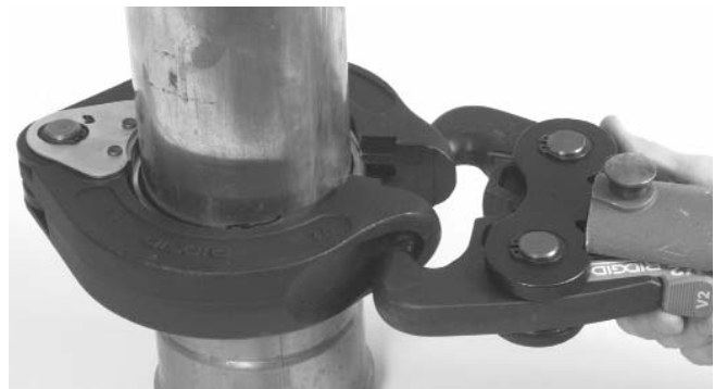
Figure 14B – Placing V2 Actuator Tips Into XL-C Ring Pockets
